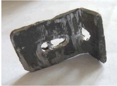
Left: Piece of lead formed and drilled to fit over the motor spindle and securing bolt at the front end.
