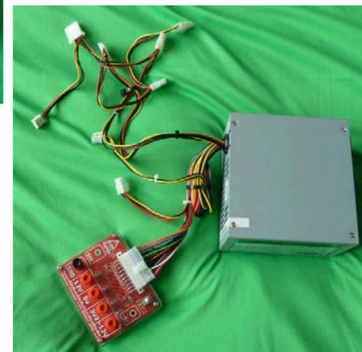
When you buy the Breakout Board you do get a 5 Watt 10 Ohm power resistor. This is for use with older ATX units that need a load on the 5 volt pin to stabilise the voltage. You are advised not to fit this unless needed. When running the resistor gets hot and therefore increases the risk of fire. All the output rails are protected by automatic resetting poly fuses.
