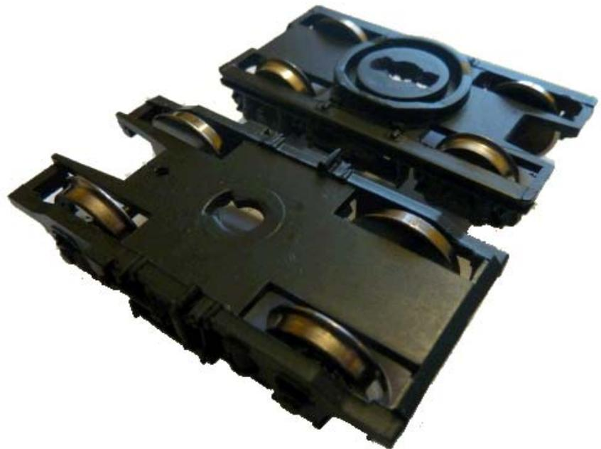
What needs to be added is a washer to sit over the raised boss on the coach chassis. I used a standard DIY store M6 washer which is just under 1mm in thickness. This will then allow the coach body to sit at the correct height above the replacement bogie. Without a washer in place the coach will derail as soon as it comes to a deviation in the track. This is because the coach body catches the top of the bogies thus restricting the coaches ability to articulate.
