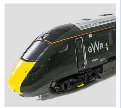
mode trains. This means they can run either on their diesel engines or by the overhead catenary. Their diesel engines are MTUs—and we know where they had their railway origins. A clue is on the front cover.
