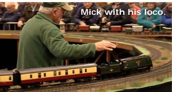
It is a meths fired live steam loco with the correct three cylinders (but without the chain driven valve gear).
