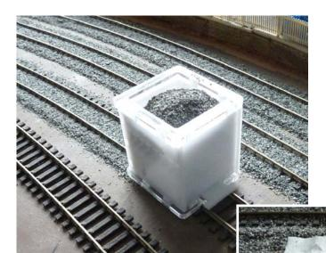
The ballast dispenser in action. You will note that in the sidings the track has not been laid on cork. The reason being that it seemed unnecessary.
