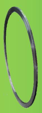
In a nutshell a Gibson Ring is basically a circlip. This is used to hold the tyre on a railway wheel. To put a tyre on a railway wheel, the tyre is heated to make it expand. While still hot it is slid over the wheel body and then Gibson Ring is sprung into the recess in the back of the tyre. To hold this in place the back of the tyre is rolled down to crimp the tyre in place. As the tyre cools it contracts thereby gripping around the wheel body.
