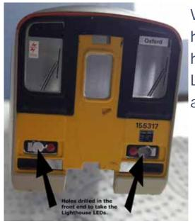
With the Sprinter body removed, two holes need drilling through the headlight moulding to take the two LEDs. These are marked by the black arrows on the image.
