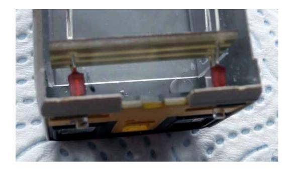
This image shows the copper strip board inside the sprinter. I found that it did NOT need gluing in place, as the projections on the LEDs pushed through the lighting apertures drilled in the Sprinter body, held it in place. Also you may need to remove the board at a future point if you need to replace a LED.
