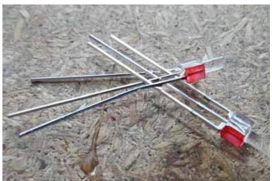
The main thing to be aware of when you use these type of LEDs is that the Anode (+) has to be common because DCC switches its functions via the Cathode (-). You will need two 1K ohm resistors. These go in series with the anode.
